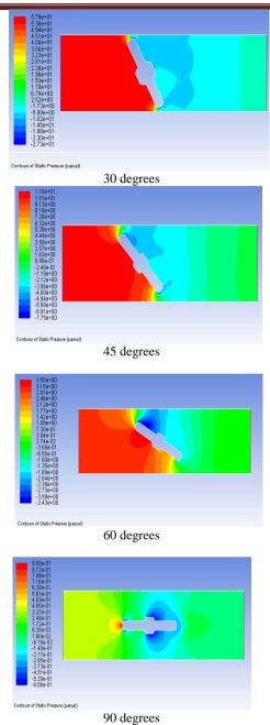
Fig. 1 Pressure plots of the different throttle opening positions
